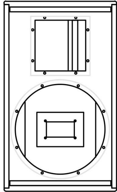
Equipped with one 12" speaker from Lavoce Italiana in a tuned enclosure. The HF section features one 2" compression driver from Celestion coupled to a diffuser, offering a dispersion of 90°x50° (H x V).
